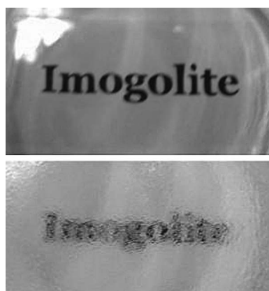
Fig. 5 The transparency of the in situ synthesized nanocomposite (upper) and blend (lower) films with imogolite : PVA = 1 : 20. The thickness of the films is ca. 100 μm. Reproduced from ref. 12b. Copyright 2005 Royal Society of Chemistry.
