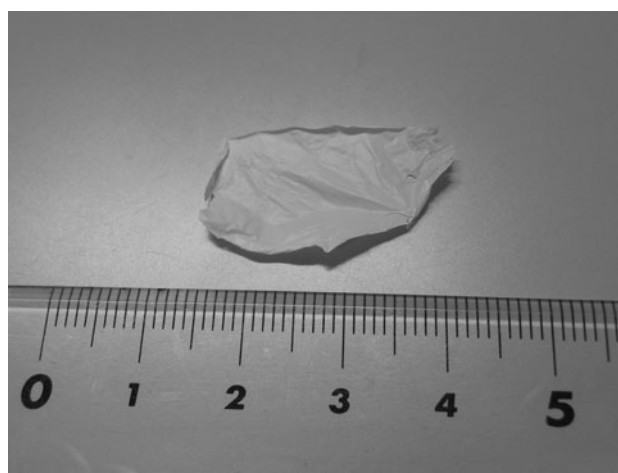
Fig. 2 A view of the precursor nanofiber mat heated at 500 °C
