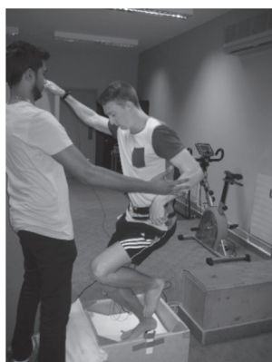
Fig.2c Setting for surprised landing White false floor is falling down
