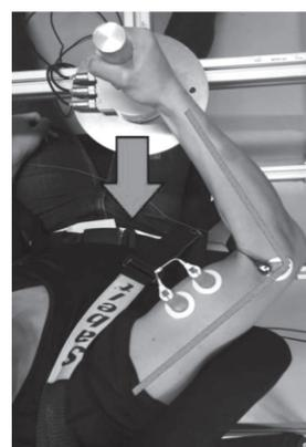
図9 Measuring equipment for output force (top view)
