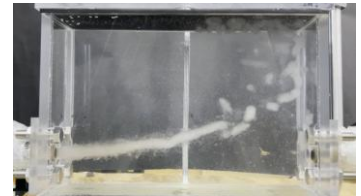
Observation of ice slurry transportation
