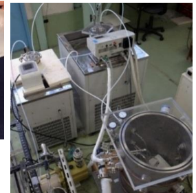
Absorption ice slurry generator made by students
