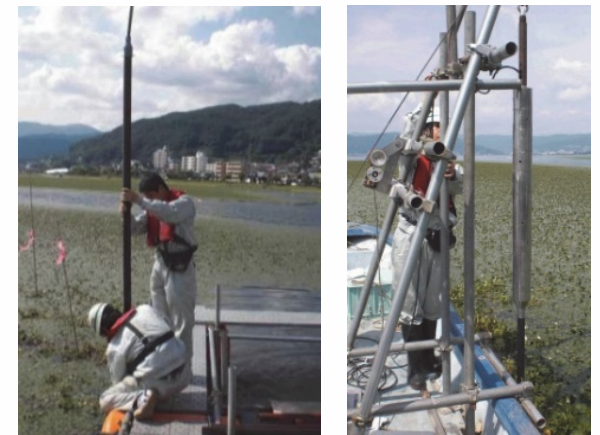
Sampling of bottom sediments in enclosed water areas (Suwa Lake), surveys of strength of lake bottom ground and density log.
