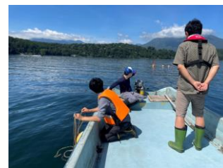
Field survey in Lake Nojiri, Nagano, Japan. A logger is installed at the center of the lake to measure dissolved oxygen and water temperature every five minutes.
