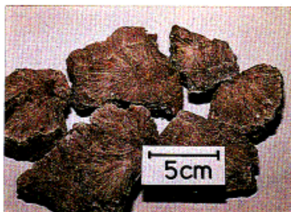
Radial type of calcarious mudstone at site No. VI. Magnifying photo. of wedge formation (Radial type).
