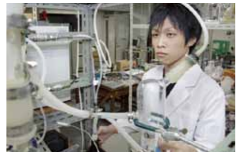
A student analyzes the process of absorbing CO 2 using a hollow fiber membrane to compare its effectiveness. Students designed the absorption and diffusion device themselves and carry out their own experiments.
