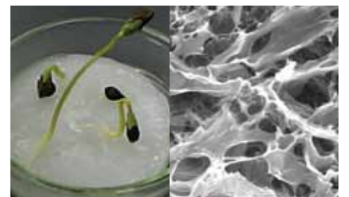
An electron microscope is used to analyze the fine structure of a water-soluble polymer gel sheet designed to facilitate seed sprouting and growth to assist in afforestation of arid regions.
