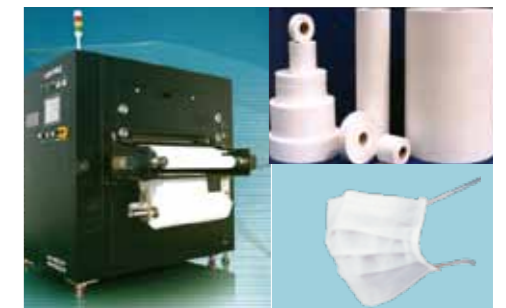
The world's first successful device for mass-producing nanofiber (left) A nanofiber separator (upper right) and a high-performance mask capable of filtering out PM 2.5 particles (lower right)
