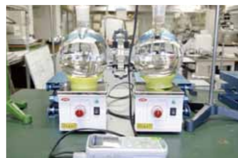
Salt water can be seen on the left and pure water on the right. A salinometer is being used to measure how much salt passes through the film to the pure water side.
