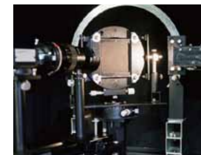
This device measures the distribution of light reflected from fabric to quantify impressions felt by people about characteristics such as depth and brilliance, allowing the beauty of cloth to be quantitatively evaluated.
