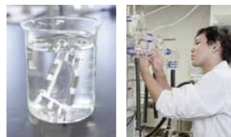
Cellulose acetate is boiled in ammonia to examine polymer changes.
