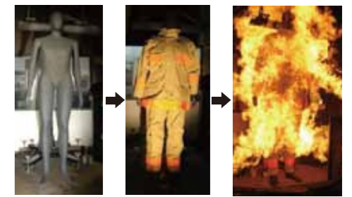
Evaluation of firefighter clothing by flash fire manikin. Fundamental research on test method against heat and flame will be contributed to international standard (ISO) development.
