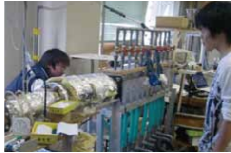
My lab is working to develop a high-performance cleaning system that instantly removes dust, contaminant gases, and foul-smelling components from the emissions of factories and garbage collection facilities.
