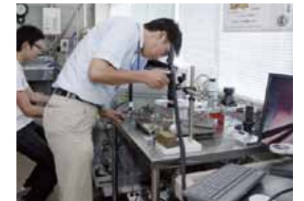
An organic semiconductor material developed in the research lab is melted and applied to a circuit board to create a transistor. We are carrying out research to create example uses that leverage its properties.
