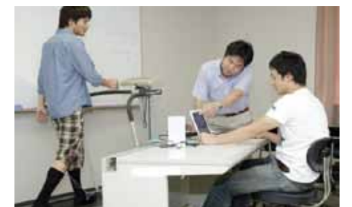
Researchers measure the changes in clothing pressure from socks using a treadmill. Comfort is quantified by measuring changes in pressure by placing pressure sensors on the feet, yielding data for later analysis.
