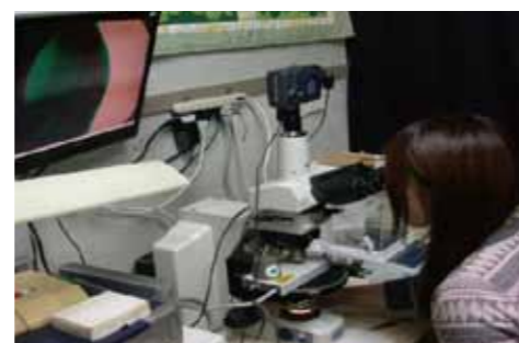
A student observes the texture of her synthesized discotic liquid crystalline semiconductor with a temperature-variable hot stage and a polarizing microscope.
