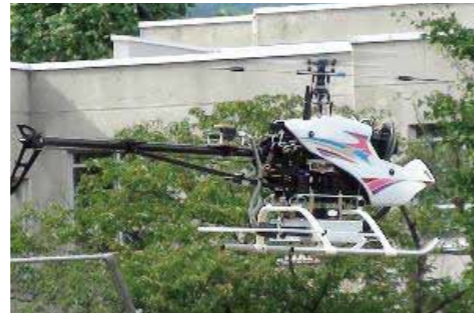
This autonomous, small-scale unmanned helicopter, one of our aerial robots, can fly without human operation using autonomous control technology.
