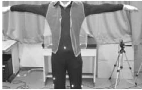
The movements of a person wearing clothing are measured using a motion-capture device (a device used to record human motion).
