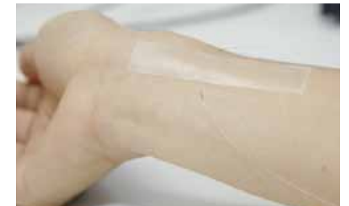
The optical fiber used to measure vital signs is so fine that it's easy to forget that it is in contact with your skin. This approach entails none of the pain normally associated with drawing blood.
