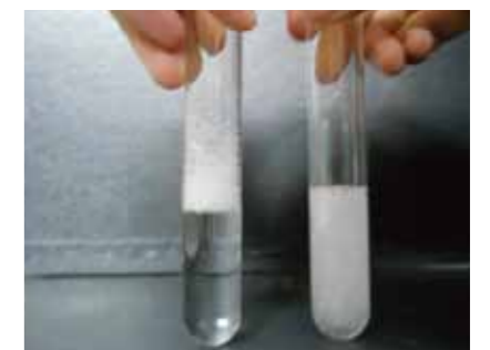
Immediately after adding a small amount of a weak alkali to an aqueous surfactant (detergent) solution, bubbles disappear and solids (hydrolyzed product) precipitate.
