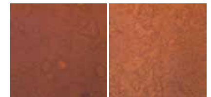
It may be possible to create materials with a variety of properties by controlling the polymer-blend structures such as sea-island structures (left) and bicontinuous structures (right).
