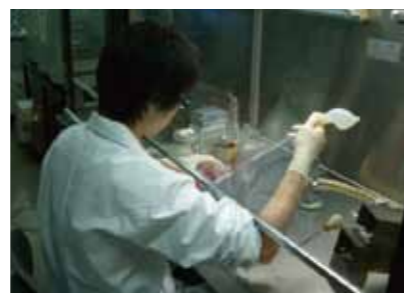
Tissue cells are cultured over a long period of time using a petri dish whose bottom is coated with the material we created, and then they are kept in a device that maintains sanitary conditions so that we can examine their functionality.
