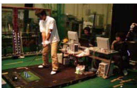
A student tests freedom of motion while wearing golf apparel. Three-dimensional motion analysis is performed using markers on the arms.
