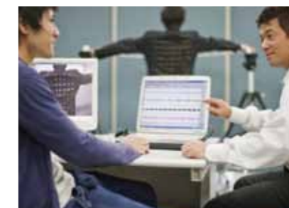
By measuring (via electromyogram) the muscle activity of a person wearing a suit, it is possible to evaluate how much freedom of movement that suit affords.
