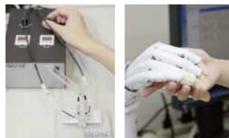
Artificial muscles that move in the same way as human beings are one basic technology for robotic hands.
