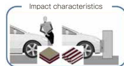
My lab is working to develop a hybrid super-fiber and carbon-fiber FRP structure that exhibits excellent buffering properties and impact strength.
