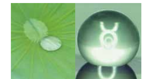
Lotus leaf and superhydrophobicity expressed by nano-periodic structure on a solid surface.
