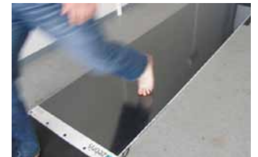
We use a pressure board—a pressure measurement sensor array with a resolution of 5 mm and 200 Hz—to investigate mechanical characteristics of walking behavior of humans and animals.
