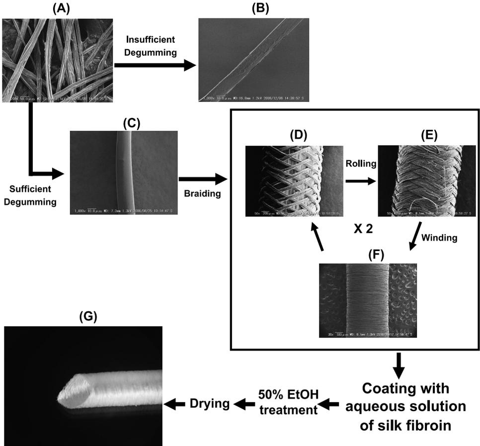
**Figure 2.** Scanning electron micrographs of silk fibers and silk grafts at several processing stages. (A) Raw silk, (B) a silk fibroin fiber after insufficient degumming, (C) a silk fibroin fiber after complete removal of silk sericin, (D) silk graft after braiding, (E) silk graft after rolling, (F) silk graft after winding and (G) the final silk graft.
