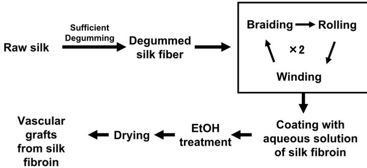
**Figure 1.** Preparation of the small-diameter vascular graft made of silk fibroin from *B. mori*.
