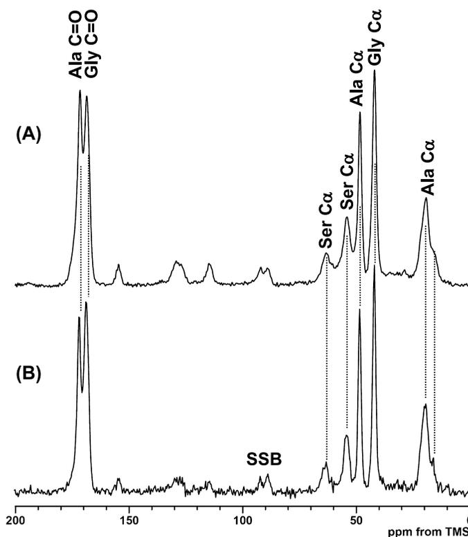
**Figure 3.**  $^{13}\text{C}$  CP/MAS NMR spectra of recombinant silk fibroin fiber from a transgenic silkworm together with the peak assignment. (A) Dried state and (B) hydrated state. SSB, spinning sideband (an experimental artifact).
