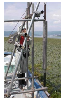
Sampling of bottom sediments in enclosed water areas (Suwa Lake), surveys of strength of lake bottom ground and density log.
