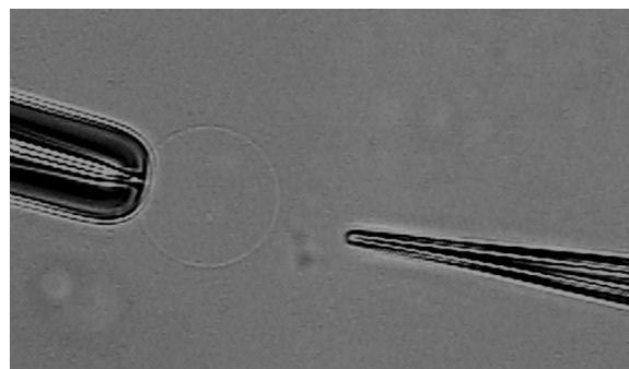
Micromanipulation of a giant vesicle. Various substances may be introduced into the vesicle by microinjection through a hollow needle.
