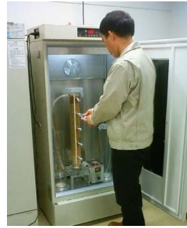
LEFT: Packed bed reactor for denitrification.
