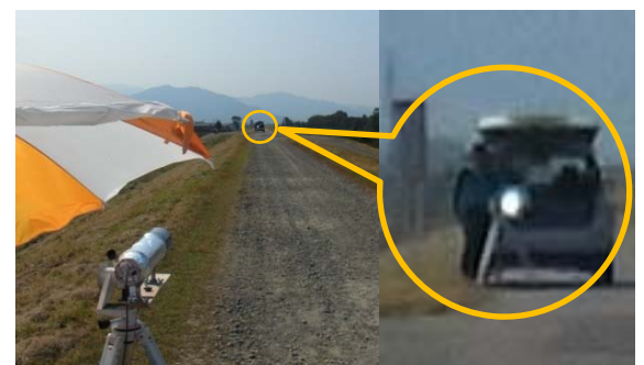
Experiment of visible light communication over long distance: The world record is 42.19km that is attained by co-working company. We are challenging to satellite communications.
