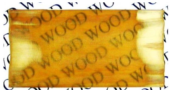
Transparent compressed wood made from Japanese cypress ( Chamaecyparis obtusa Sieb. et Zucc. ).
