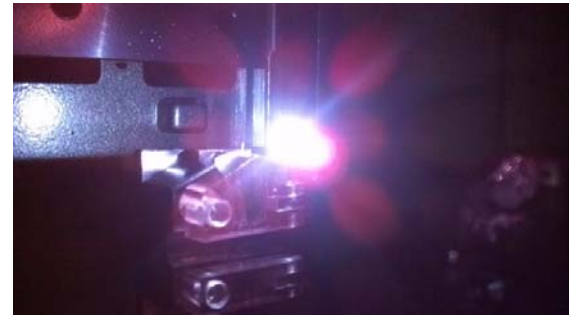
Pulsed Nd:YAG laser light is invisible; however, air is plasmarized to flash strongly because a huge amount of energy is condensed to a focal point.
