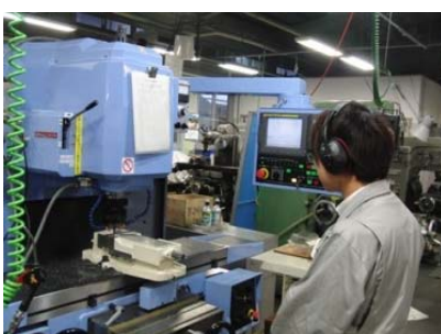
Program processing by NC milling machine for making the experimental device used for a graduation research project.
