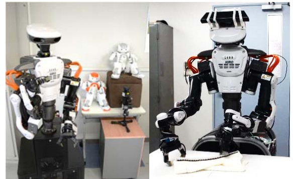
Left figure: our research platform (robots). A life-sized dual-arm robot and small humanoid robots. Wheeled mobile robots are also used. Right figure: an experiment that the dual-arm robot manipulates a piece of clothing.
