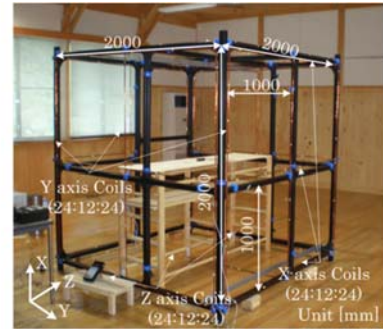
Simple-Cubic-3 coil system for generating uniform magnetic field to three dimensional direction. It is used for demonstration of several magnetic field environment.
