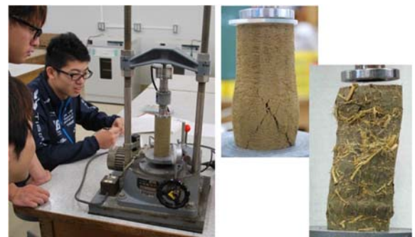
Experiments in the class by third year students (left); destruction of material composed entirely of soil (upper right); strength is improved significantly if paddy-rice straw is mixed with it (lower right).
