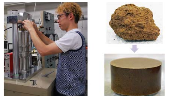
Loads exceeding several tons are applied to clay taken on campus (upper right) to reproduce super hard clay existing several hundreds of meters below the ground (lower right).
