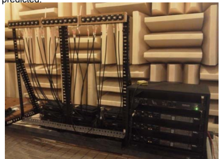
Loudspeaker array system installed in an anechoic chamber, a room without any reflected sound from the walls.
