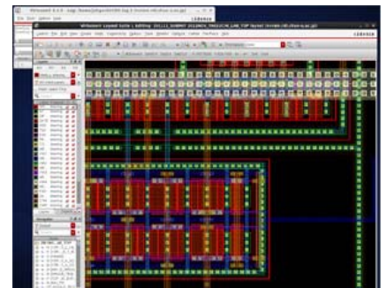
Students define the specification and design a circuit. To fabricate a chip, a circuit designer draws a layout with nm-order scale by CAD software.
