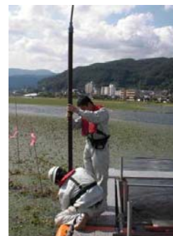
Sampling of bottom sediments in enclosed water areas (Suwa Lake), surveys of strength of lake bottom ground and density log.
