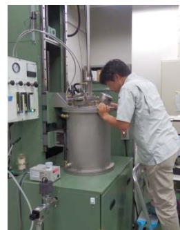
Left: An operator is observing the inside of the Czochozralski growth furnace. Right: A germanium single crystal grown from the melt.
