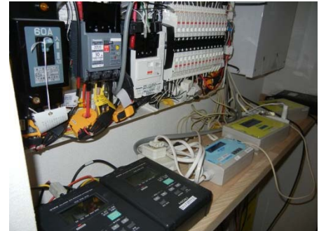
Equipment to measure the amount of electric consumption and electricity generated from fuel cell co-generation systems and photovoltaic power generation systems.
