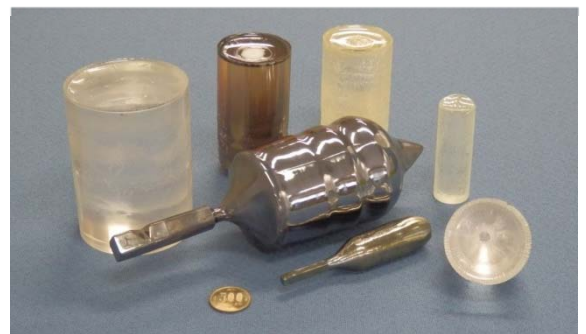
Several typical single crystals, such as silicon (center) and sapphire (left and right side), grown in our laboratory or cooperative companies.
