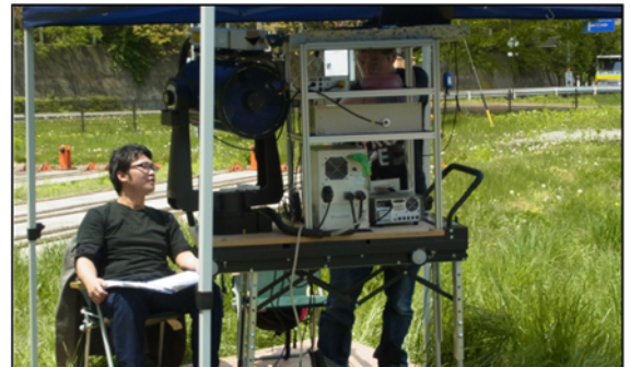
LIFS (laser-induced fluorescence spectrum) lidar field work: Remote sensing of living environments such as air-borne pollen, bio-aerosol, water quality, plant growth status, and others.
