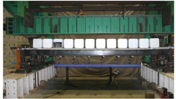
Experiments and numerical analyses investigating lateral buckling of large-span composite beams subjected to live loads
