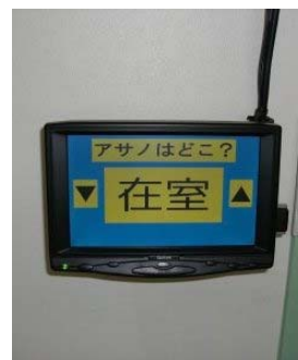
Location display system using an LCD touch panel
