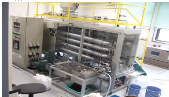
Continuous flow-type hydrothermal reactor we designed: this is a powerful tool for processing organic substances from plant biomass.
