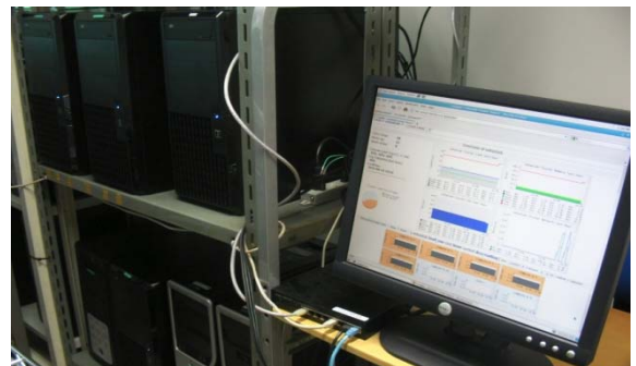
In order to simulate wireless systems, we build a PC cluster with which many PCs can be virtually viewed as a high spec computer.
