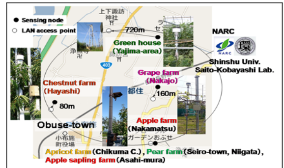
An agricultural sensing network system (AgriServer) operating in Obuse-town: Information on products growing in the fields are provided through the "Nou-Live" website.
