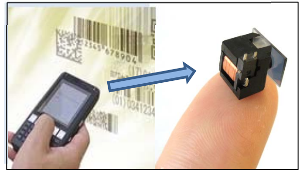
Micro resonant motor as a barcode scanner for a smart-phone device.
