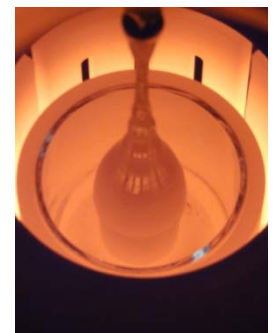
Left: An operator is observing the inside of the Czochozralski growth furnace. Right: A germanium single crystal grown from the melt.
