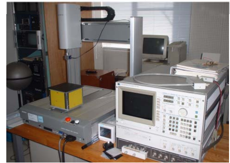
Robot arm and impedance analyzer using the contact experiment
