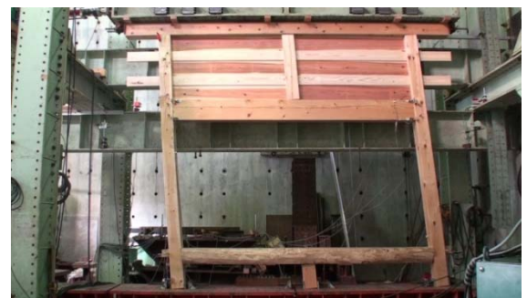
Static loading test of the wood frame of traditional construction houses in the Gassho style of Shirakawa-go
